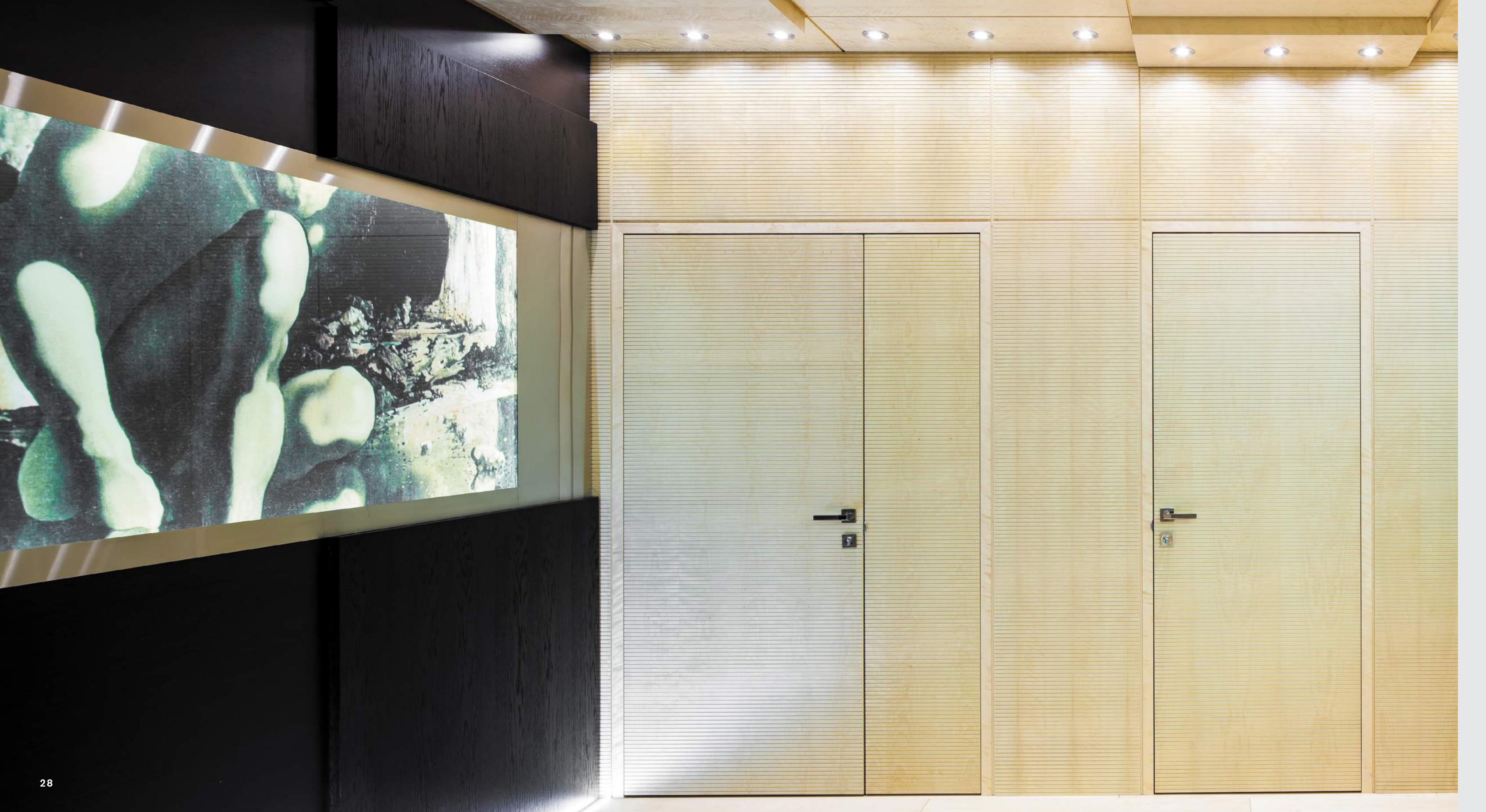
The acoustic comfort is reached by using selected materials for solid wall panels and for doors. Visible elements of wall frames can be retrofitted and be made identical to walls.
